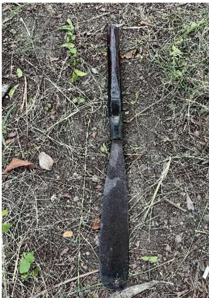
Figure 1. "Tagad" – a traditional digging tool used for excavation.
