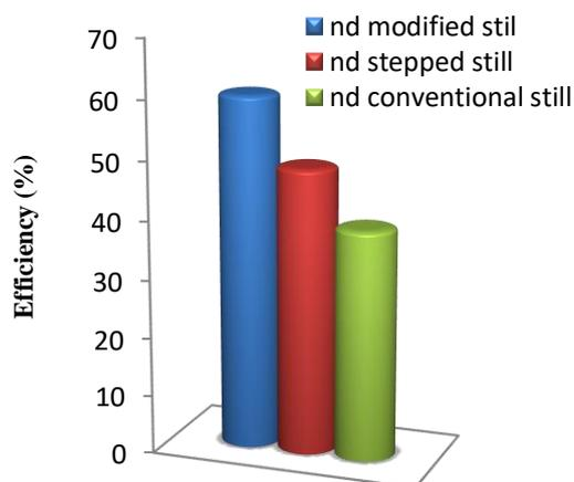
Figure 6: The daily efficiency of modified stepped solar still, stepped solar still without modification and conventional solar still.
