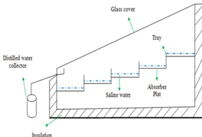
Figure 2: Schematic diagram of Stepped solar still without modification
