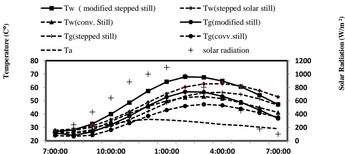
Figure 4: The hourly temperature variation and solar radiation for modified stepped solar still, stepped solar still without modification, and conventional solar still
